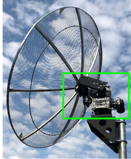
Az/El motors + position sensors
