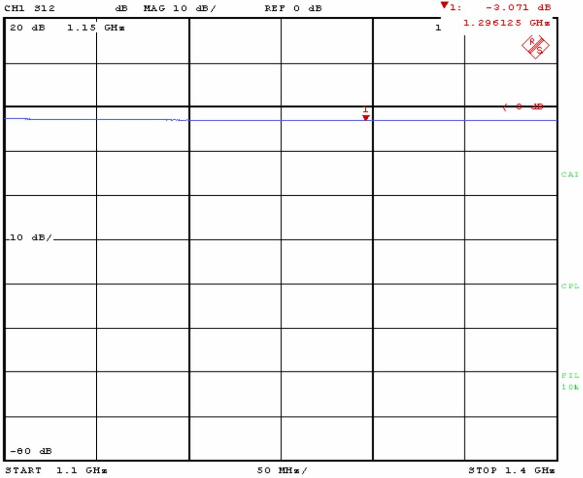
Phase balance between output port 3 and output port 4 (180 dgr)
