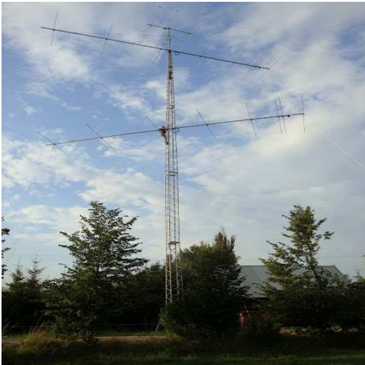
Photo.3 2 x 28MHz antennas on the station SP8CUW & SP8CUR powered by Stack Match
