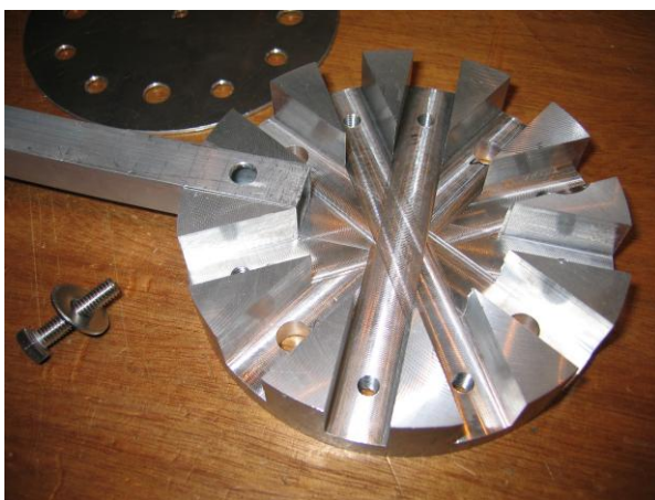
CNC milled center and easy to place rib
