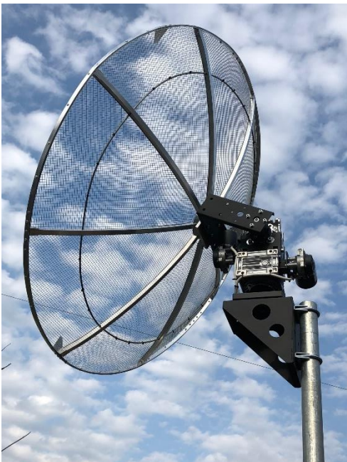
SPX-01 + PLATE-03 and 1.2Meter Mesh Dish mounted
